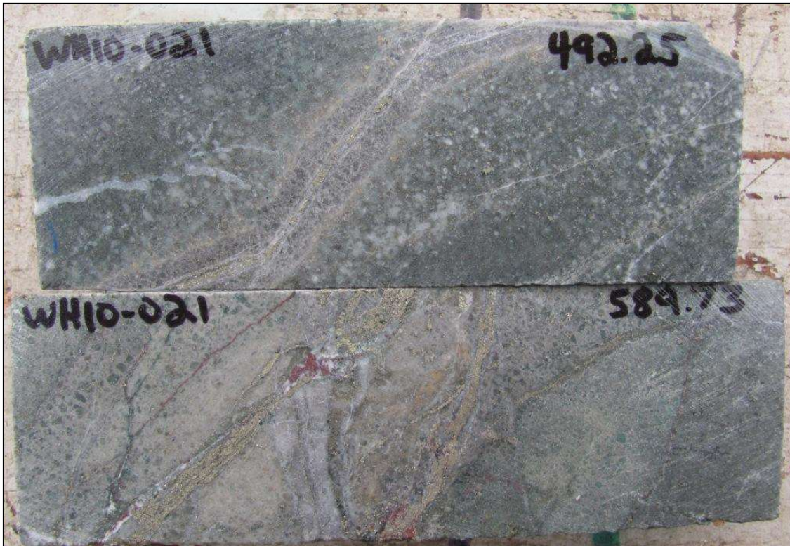
Figure 6-12 D-style pyrite veins with well-developed phyllic halos (Whistler Deposit), that cut and off-set B-style quartz veins (lower sample). Also note the local occurrence of hematite at the intersection of both vein types (magnetite>hematite?)
