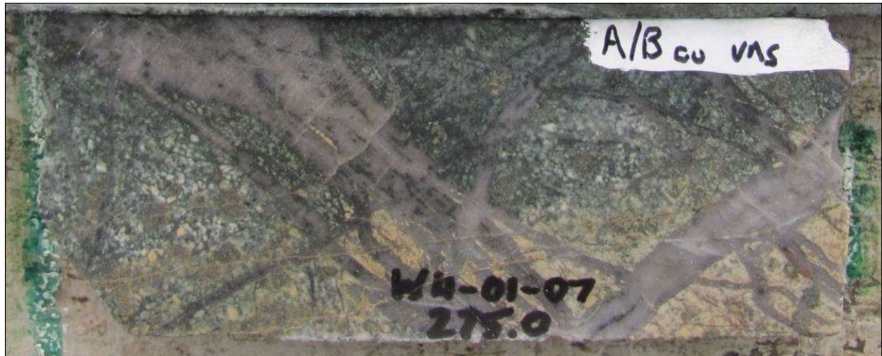
Figure 6-11 Photo of chlorite-sericite (+calcite) alteration overprinting potassic – magnetite alteration in a zone of quartz vein stockwork, subsequently cut by later Dpy veinlets with sericitic and iron-carbonate halos (Whistler Deposit)
