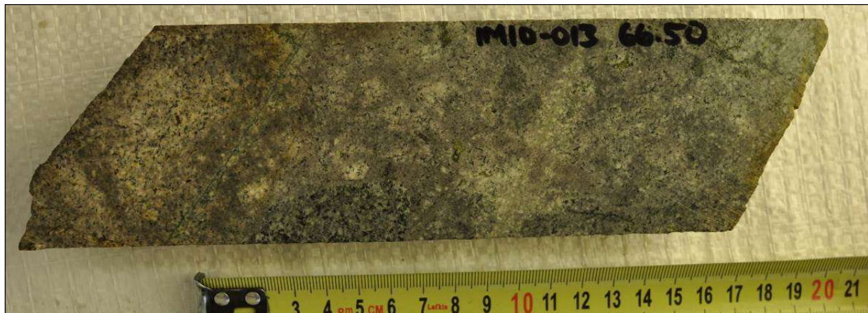
Figure 6-18 Photo of monzonite-matrix intrusive breccia with patchy albite alteration, silicification and disseminated chalcopyrite
