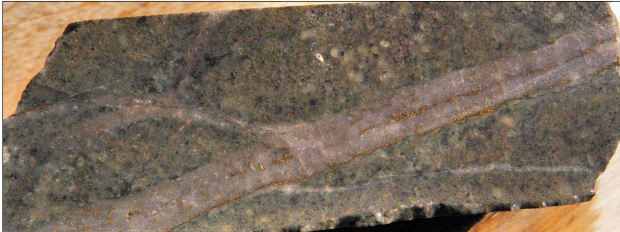
Figure 6-10 Photo of a classic B-style quartz vein with a chalcopyrite-filled centreline cutting an irregular, wormy A-style quartz vein (Whistler Deposit, WH 08-08, ~123.0 m)
