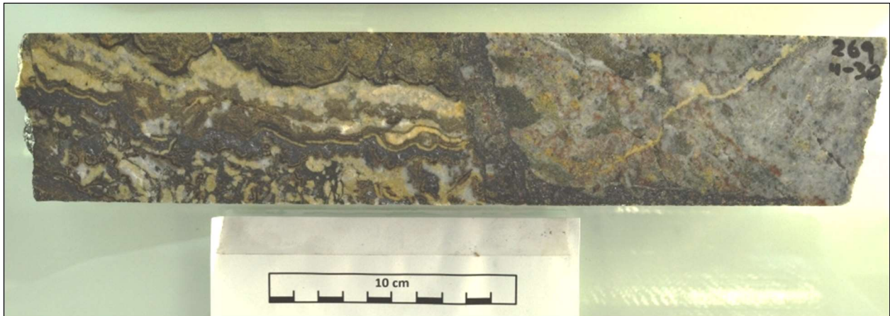
Figure 6-13 Photo of quartz-carbonate vein from Raintree West (WH11-030) showing well-developed colliform banding and coarse-grained sphalerite and galena (Source: MMTS, 2015)
