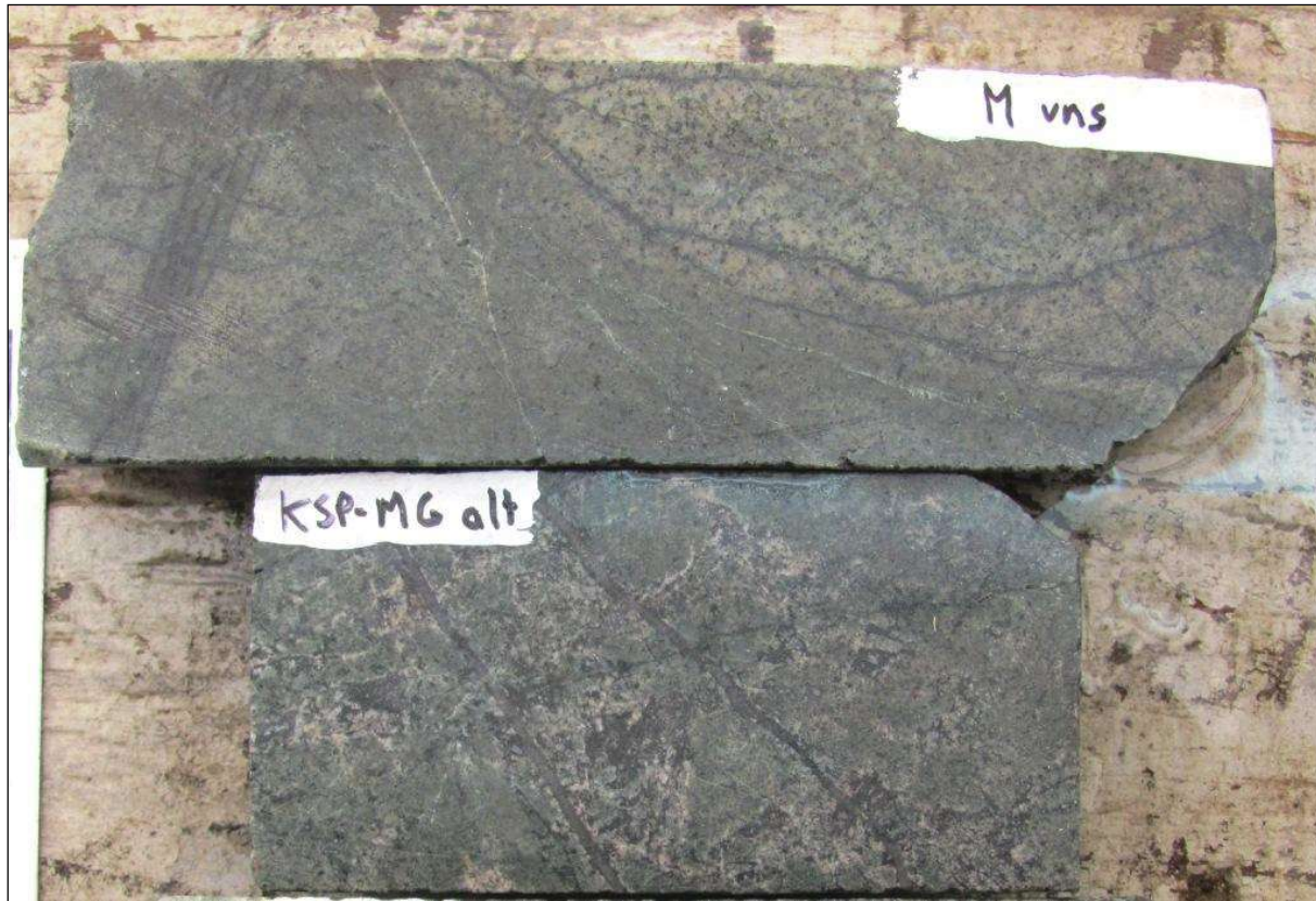
Figure 6-9 Photo of irregular M-veins in dark magnetite alteration of mafics (upper) and pervasive pink-black blotchy k-feldspar and magnetite alteration (lower) with wormy quartz + magnetite + chalcopyrite A-veins (Whistler Deposit)
