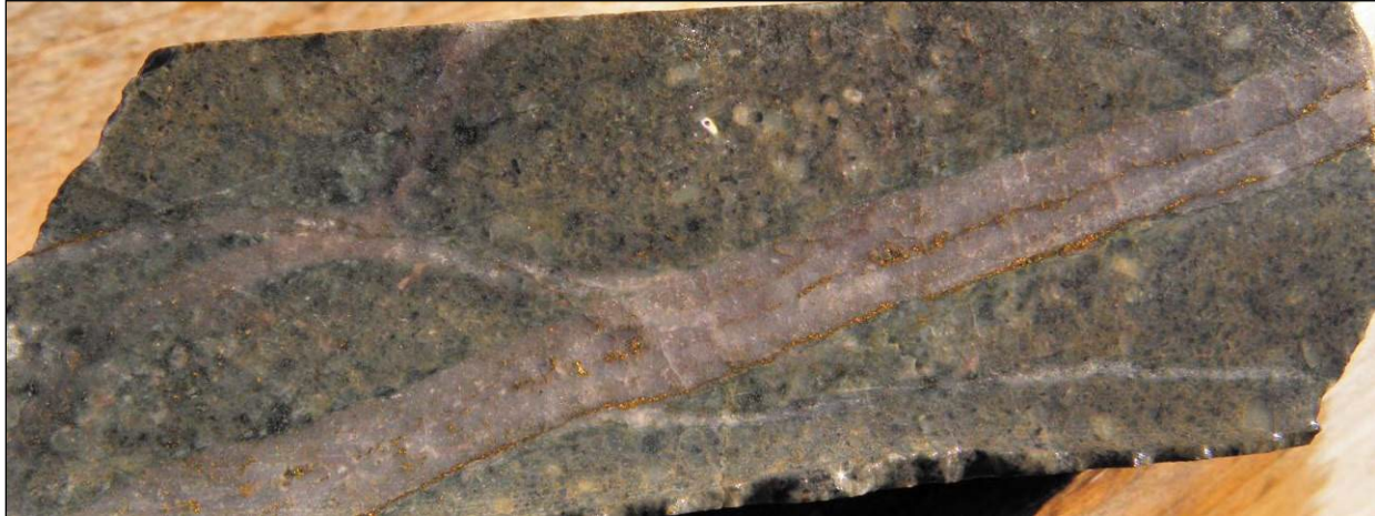
Figure 7-10 Photo of a classic B-style quartz vein with a chalcopyrite-filled centreline cutting an irregular, wormy A-style quartz vein (Whistler Deposit, WH 08-08, ~123.0m)
