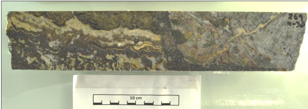
Figure 7-13 Photo of quartz-carbonate vein from Raintree West (WH11-030) showing well-developed colliform banding and coarse-grained sphalerite and galena
