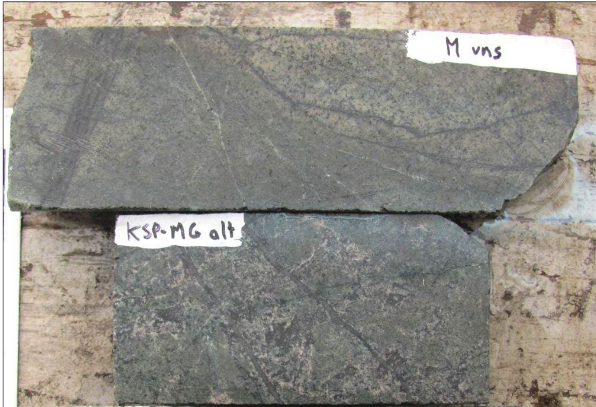
Figure 7-9 Photo of irregular M-veins in dark magnetite alteration of mafics (upper) and pervasive pink-black blotchy k-feldspar and magnetite alteration (lower) with wormy quartz + magnetite + chalcopyrite A-veins (Whistler Deposit)
