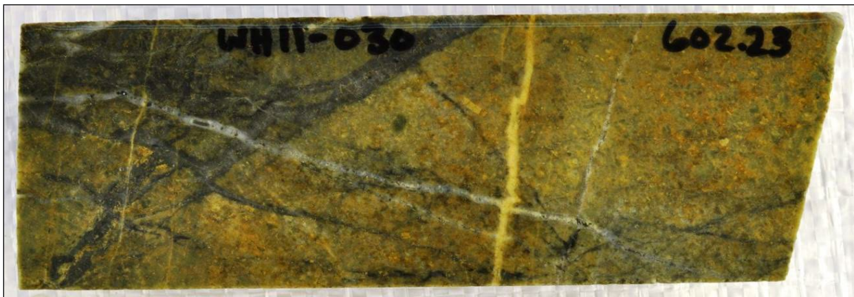
Figure 7-14 Common vein paragenesis in all porphyry occurrences in Whistler Area: dark grey quartz vein stockwork with chalcopyrite (A- and B-style), cut by quartz-calcite-carbonate-sphalerite-galena veinlet (Dbm veins, top left down to bottom right), cut by narrow Fe-carbonate veinlets with Fe-carbonate alteration halos (Raintree West example)
